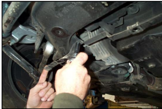
Figure 16 - Remove rear mount of belly pan, if present, with a 10mm wrench
