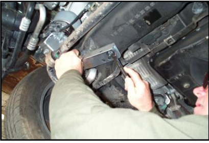
Figure 25 - With a 17mm box end wrench or socket, start tightening the greased 10mm bolt
