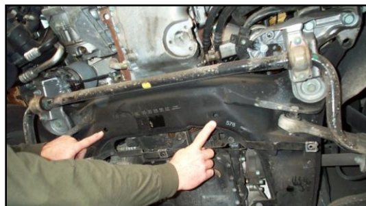
Figure 22 - Locate the two 13mm hexagonal holes in your subframe
