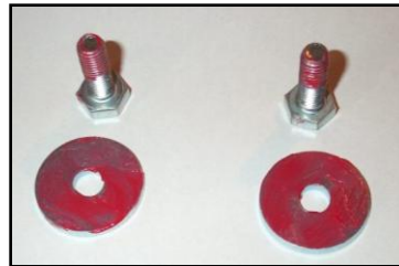
Figure 42 - Large, previously greased bolts
