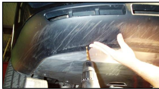
Figure 68 - Drill a hole in the spoiler and then into the aluminum skid plate
