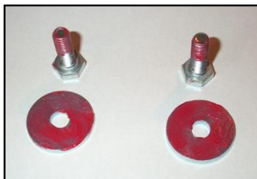
Figure 17 - Grease the threads of the provided large silver 10mm bolts
