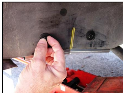
Figure 36 - Threading in the black 6mm screws
