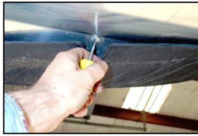
Figure 56 - Turn all Dzus 1/4 turn fasteners clockwise to their stops
