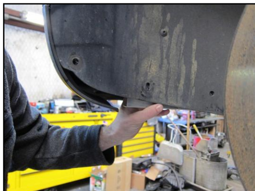
Figure 38 - Line up the holes to the speed nuts
