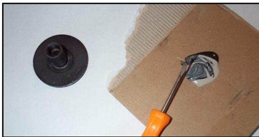
Figure 23 - Mixing 1/2 ounce of a two-part epoxy on a paperboard or plastic sheet
