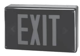
The NAV series vandal resistant exit sign is designed to stand up to high abuse areas such as correctional facilities, schools, apartment complexes, and public areas that may be subject to vandalism. The NAV features an IEC IP66 rating standard, and is suitable for wet or hose down applications.
