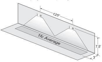
Using multiple NFT-HO units (5.4 Watts lamps) mounted at a typical 7.5' height delivers 115' on center spacing with a 6' wide path of egress.
