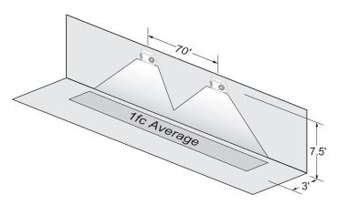
Using multiple NFT units (2.7 Watts lamps) mounted at a typical 7.5' height delivers 63' on center spacing with a 6' wide path of egress.
