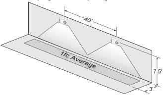
Using multiple LED-52 (2 watt) units mounted at a typical 7.5 foot height delivers 30 foot on center spacing with a 6 foot wide path of egress.
