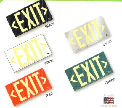
Designed for maximum durability, the Glow Maxx 50 Photoluminescent Series Exit Sign is constructed using a steel stencil face plate with rigid photoluminescent insert. Ideal for high and low level applications. Easy pop out directional chevrons. UL 924 Listed with three external charging light sources: fluorescent, metal halide, and mercury vapor.
