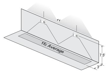
Using multiple LED-52 (4W) units mounted at a typical 7.5' height delivers 37' on-center spacing with a 6' wide path of egress.
