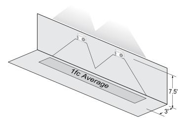
Using multiple LED-51 (2W) units mounted at a typical 7.5' height delivers 27' on-center spacing with a 6' wide path of egress.
