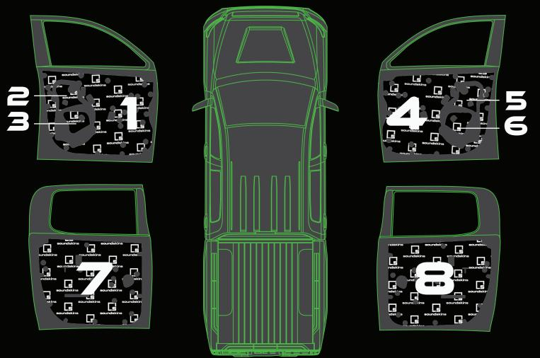
1) Driver Front Door Panel 2,3) Driver Front Vapor Barrier Pieces 4) Passenger Front Door Panel 5,6) Passenger Front Vapor Barrier Pieces 7) Driver Rear Door Panel 8) Passenger Rear Door Panel
