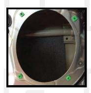
2. Wipe down the metal surfaces around and behind the speaker hole. Be sure it is clean of all debris, oil, dust, moisture, etc. and let it air dry completely. Take the acoustic wavy foam pieces and apply them onto the metal surface behind the speaker (inside the speaker hole).
