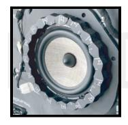
4. Trim off the excess material with scissors and connect the two ends of the strips. Your installation is complete, and you can reinstall your door panel.
