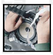
3. Then, reinstall the speaker and wipe down the trim of the speaker plate. Peel off the backing on part of a foam strip and apply the strip around the face of the speaker, peeling off the backing as you go until the entire speaker face is covered.
