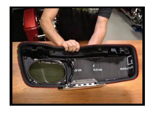
3. Panel 2 covers the bottom of the latch mechanism itself. Ensure you don't get the left and the right side pieces mixed up. Mock it up to ensure correct placement before applying.
