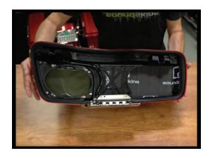
2. Next, install panel 1. There are two relief cuts on this piece that allow it to bend where it needs to on the rear and outside edge of the lid. Align this panel along the back edge of the latch mechanism and move on to the rear so everything lines up.
