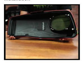
1. The first panel to go in is one of panel 4. Position this panel directly under the center of the latch mechanism bridge where you made your pencil marks earlier. This panel will keep the latch from rattling against the top of the lid. Then, reinstall the latch mechanism. Reinstall the hinge cover and ensure the lid gasket is put back in place.
