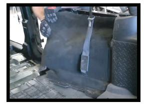
1. Start by unclipping the side panels on your wheel wells. Begin from the top of the side panels. If you have a factory subwoofer, remove the torque bolt at the front to unplug the subwoofer.
