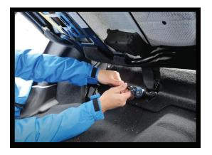
3. To remove the backseats, you will need an 18mm socket to remove the bolts. Take out the 2 bolts in the back and the bolts in front of the backseats. When all bolts are out, remove the smaller seat first, then the larger seat. Be sure you also remove the seatbelt bolts. Then, remove the carpet under the backseat area.
