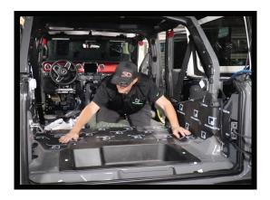
5. Start installing the kit by mocking up the wheel well pieces. There is a different between the left and right wheel wells, and you will have to unscrew some plugs on both wheel well sides. Make sure it lines up correctly before you pull the backing paper off and start rolling the material down using a roller. Make sure the material is applied evenly without no air bubbles. Use a razor blade point or household needle to release any air pockets.
