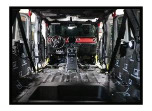
6. Repeat these steps for all pieces, moving on to the main trunk floor piece, then the smaller floor pieces. After all pieces are installed, double check that no holes are blocked for the mounting hardware and all the material has solid contact. Last, replace the carpet, seats, and panels and tighten all the bolts securely.
