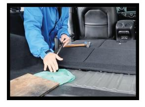
2. Next, unclip the flap/panel that sits on the back of the backseat. It will be tight, so use a clip removal tool or the back side of a hammer to wedge the clips out. Once this panel is off, it will reveal the 3 bolts holding down the backseats of the Jeep.
