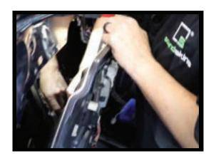
3b. To prop the windows up for JKs, remove the 10mm bolts around the plastic insert and disconnect the wire harnesses. Peel the panel back and pull the toward you. Then find the alginment pin located between the insert and door connected to the bottom of the glass and disconnect it from the glass. This will allow you to slide the glass up. Prop the window up with a rubber wedge covered by a microfiber cloth.
