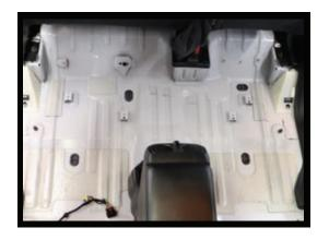
8. Once you clear seats, can start working up the carpet. It will be a bit more difficult because it's molded to the floor. Remove the carpet completely and lay it down on a flat surface in order to not damage integrity of the material. Now wipe down the floorboards as you did the door panels (you may need a vacuum depending on how dirty your floors are). If you wish, you can also remove your door seals.
