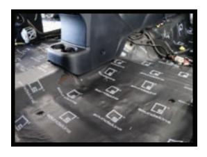
11. The largest piece will be easier to install if you have help. It will be the rear section and it comes in one large piece. Start with one side and roll it down from one side to the other.
