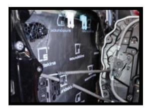
5. Locate the piece of the kit with the label on the back that coincides with the door you're working on. Make sure it lines up and is correct before pulling the white cover paper off, then pull off the white paper and start placing the material at the top and work your way down. Use a roller to apply the material completely. Use a razor blade point or needle to release any air bubbles. Repeat these steps for all door panels, then reverse the process to replace your doors.
