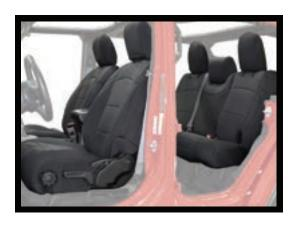
7. Remove the front seats and the carpets. Use the appropriate size socket set. There are four bolts per front seat - remove the yellow electrical seat plug and then remove the seats, being careful not to scratch the seats against your car.
