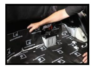
12. For Gladiators, there will be two extra pieces to install in the rear section. Find the label that coincides with the floor section and roll the pieces down.
