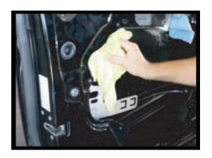
4. Note that the plastic inserts do not need to be completely removed to install the door pieces, you can simply hold it off to the side or have a friend help as you install the material. Now you are ready to prep the metal surface with a microfiber cloth and Acetone (use a breathing mask). Wipe away any moisture, oil, debris, etc. Then let air dry. The point is to get the surface clean to ensure material glue contact.
