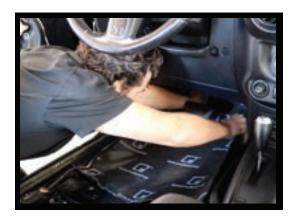
9. Start with the front pieces and find the label that coincides with the floor section. Make sure to check it first to ensure that it fits in the designated area. Once confirmed, pull the white paper off and apply the material with a roller, starting from one side and working the material back.
