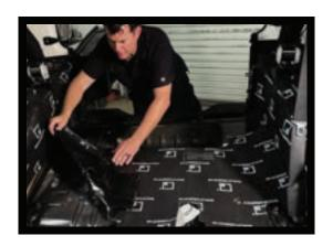
6. Move on to the floor pieces starting with the main floor piece. Mock the piece up before applying the material. We suggest folding the material in half crosswise and peeling off half of the backing. Once you installed one side, peel the backing off the other side and install the rest of the piece.
