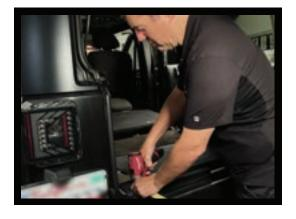
1. Start with a T-30 torx bit to remove all clasps that hold the carpeting down. Remove the hard panel that goes over the center tub, then remove the pastic tub located over the drain hole.
