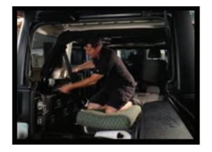
5. Start installing the kit by mocking up the wheel well pieces. Make sure the pieces up correctly before you pull the backing paper off and start rolling the material down using a roller. Make sure the material is applied evenly without no air bubbles. Use a razor blade point or household needle to release any air pockets.
