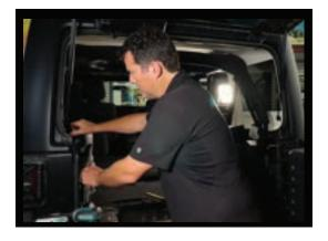
2. Using a panel tool, snap off the plastic panels that go behind the wheel wells and pillars (on top of the roll cage). There is a 10 mm nut on the backside of the panels. Use a wrench or socket tool to loosen it in order to slide out the plastic panels.
