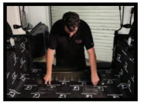
7. The final piece goes in the trunk tub. Mock it up to ensure the piece is right side up before installing.
