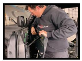
2. Pull the door panel away slowly. There will be 2 plug clips that will need to be released as well as a wire plug to disconnect. Set the door panel aside and unhook all plugs, remove the vapor barrier, and clean the car metal surface using a microfiber cloth and Acetone or other cleaning solution. The point is to get the surface clean to ensure material glue contact.
