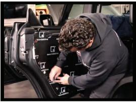
3. Now, apply the door pieces. Peel off the backing paper starting at the top, tack the piece onto the door and work your way down, pressing down the material and pulling down the backing paper more as you go along. Feed the harnesses through the proper holes and ensure everything is aligned before pressing the entire piece down. Repeat steps 1-3 for all doors. Then replace your door panels and reconnect the wires and enjoy your quiet new ride!
