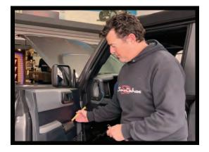
1. Start by locating the fastening hardware on the door panels. There will be one behind the door handle under a plastic cover, one behind the door grab handle that you will have to pop out to reveal, and 2 at the bottom right corner of the door panels. Take a 7 mm socket and remove. Then, use a panel tool to pry the panel off the door, start from the bottom right corner. Be sure not to break any clips or mounting hardware.
