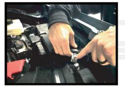
1. Start by disconnecting the negative terminal of your car battery with a 10mm bolt. Loosen it up and ensure it is not touching the battery - you can place a rag in between the bolt and the battery.
