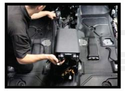
16. Locate the two 7mm bolts on the top and bottom sides of the center console covered by plastic keepers and remove. There are also a pushpin in the center of the right side that can be slid out with a pry tool. Remove these bolts and take out the final piece of the center console. There will be one harness to unplug upon removal.
