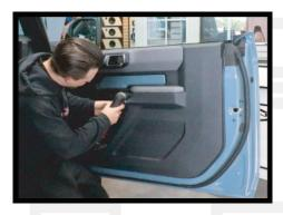
2. Locating the fastening hardware on the doors. Use a panel tool to release the plastic cover on the grab handle, which will reveal two 7mm screws on each side. There are three 7mm's at the bottom of the door panel, and one behind the door handle under a plastic cover.
