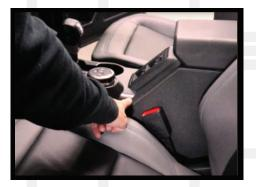
13. Then, use a panel tool to lift up the center console main top piece. It will unsnap through the seam area as seen in the photo to the left. Unplug the harnesses and set the piece off to the side.
