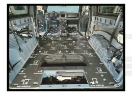
20. After all the pieces are installed, double check that none of the holes are blocked for the mounting hardware and all the material has solid contact. Then, reverse the disassembly process – replace carpets, center console, bolts, seats, plugs, etc., reconnect the battery, and enjoy your quiet new ride!
