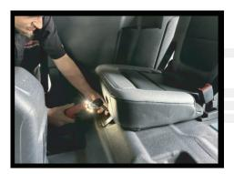
8. Next, move to the rear seats. In the trunk, remove the trim covers on the seat back rear mounting hardware. Then, move forward to remove the seat cushions using a Torx fastener to remove the bolts on the mounting hardware underneath. Remove the bolts in front of the rear seats, and remove the rest of the rear seats. Now move back to the trunk and remove the 18mm bolts on the sides of the seat backs and in the seatbelt mounts.
