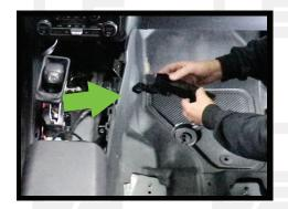
15. There will be a black plastic keeper crossing over the top of the center console held by 7mm bolts. Remove this piece.
