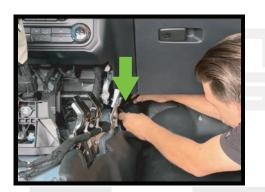
17. Unbolt the seatbelts from the floors and remove the carpeting which loops around the top of the center console and can't easily be removed. You have 2 options:
