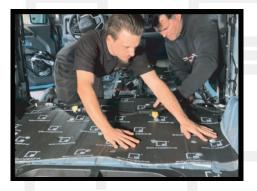
19. Now, install the floor pieces by peeling back one small section of the piece, aligning it with holes and plugs, tacking it in place, and working your way down, pulling the backing paper off as you go and ensuring proper alignment before pressing the material down firmly. Some pieces may require wire harnesses to be lifted up in order to be installed. Repeat with all floor pieces.
