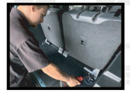
7. Move on to the trunk area. Remove the bottom plastic door seal by pulling it up, and pop up the lasso hold trim covers on all four corners of the floor. Each trim cover will reveal two 10mm bolts holding down the lasso holders. Unbolt and remove these to take out the trunk flooring.
