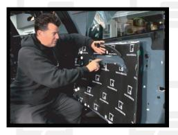
4. Now, apply the door pieces. Peel the backing paper off a few inches at the top, center the material around the holes and plugs, ESPECIALLY the large hole around the area of the door that is exposed while the door panel is on, then tack the top of piece onto the door. Pull away the paper little by little as you continue rolling the material down. Feed the harnesses through the proper holes and ensure everything is properly aligned before rolling the piece down fully. Repeat for both doors.
