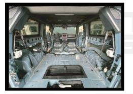
18. Clean the floor metal surfaces with a microfiber cloth and Acetone or other cleaning solution and let it air dry.
