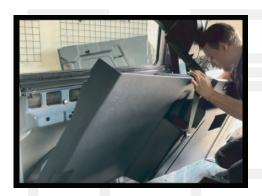
9. Move on to the side panels. These panels can be popped off easily by pulling them out. Unplug the panels and set them aside, then head to the cabin to remove the center console.
