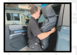
5. Now, remove the front seats. There are four 13 mm bolts holding down the seats, some are covered by trim cover plates on the mounting hardware. Then, disconnect the harness under the seat by sliding the red security tab out of the way and pinching the connector. Carefully remove the seats.
