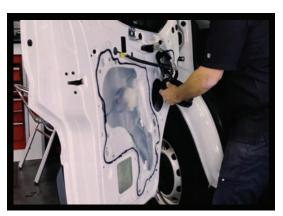
3. Next, remove the vapor barriers, unscrew and disconnect the speakers, and unclip the speaker wire keeper from where it is attached on the door's metal surface. Clean the car metal surface thoroughly with a cleaning solution such as acetone or alcohol and a microfiber cloth. Now the kit is ready to be installed.
