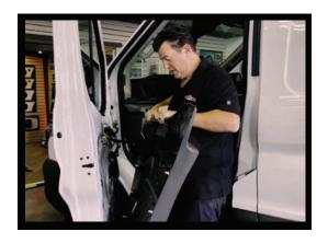
2. Remove the red reflector on the outer side of the panel by pushing it toward the outer side (away from the vehicle). It will be tight. Then, remove the 7mm bolt underneath the keeper. Once everything is off, use a panel tool to unsnap the door panel. Hold the door panel up, release all plugs and cables, and remove the door panel completely.
