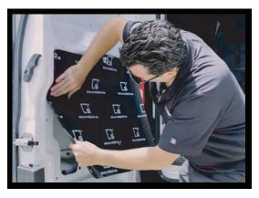
7. Then, peel the backing paper off the top section of the kit piece. Align the top of the piece with the door holes and ridges, pressing the section down once it is correct. Then, remove the rest of the material, rolling the material down from the perimeter of the doors first, then work your way inward. Once you are done, replace the door panels by pressing them into their correct plugs.
