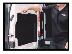
6. Now, move on to the rear doors. First, use a panel tool to wedget into the areas between the door panel and door to unsnap the door panels. Remove the vapor barriers and clean the car metal surface thoroughly.
