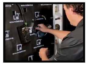
5. Press down onto your car speaker hole area, feeling for the speaker wire. Use a razor blade to cut around the speaker hole, being careful to not cut the wire harness. Take this cut out and apply it behind the speaker hole on the outer door skin to act as a backwave. With a blade, score the material where the wire harness is and tuck the harness between the two flaps.
