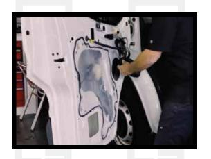
3. Next, remove the vapor barriers, unscrew and disconnect the speakers, and unclip the speaker wire keeper from where it is attached on the door's metal surface. Clean the car metal surface thoroughly with a cleaning solution such as acetone or alcohol and a microfiber cloth. Now the kit is ready to be installed.
