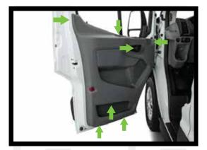
1. Start by removing the front door panels. Locate the keepers that hide the door hardware. The keepers will be a combination of 7mm and T-20 torx bits. There is one on the top outer corner, in the door grab handle on top, in the door release, in the door cubby on the upper inner side, one on the top side of the cup holder, and two 7mm's under the door panels.
