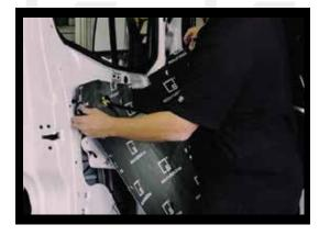
4. Peel off the backing paper from the top section of the kit piece to start. Then, take the door cable and put it through the large hole at the top, and center the kit piece around the door plug holes to ensure proper placement before pressing the top of the piece down. Then, remove the rest of the backing paper, feed the cable through the large hole on the inner side of kit piece, and use a roller to apply the rest of the kit from top to bottom, ensuring the piece aligns with the holes.
