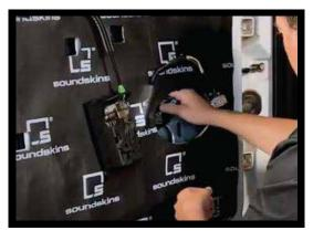
5. Press down around the speaker hole area. Use a razor blade to cut around the speaker hole, being careful to not cut the wire harness. Take this cut piece and apply it behind the speaker on the outer door skin to act as a backwave. Then, score the material where the wire harness is and tuck the harness between the two flaps. Reinstall your speaker, replace the door panels and plug the cables back in. Repeat steps 1–5 for both front doors.
