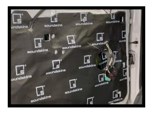
5. Press down firmly onto the area where your car speaker hole is, and feel for the speaker wire. Use a razor blade to cut around the speaker hole, being careful to not cut the wire harness. Take the piece you just cut out and stick it behind the speaker hole on the outer door skin to act as a backwave. Score the area where the wire harness is with your blade and tuck the harness between the two flaps. Plug in your speaker.
