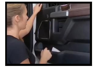
1. Start by locating the fastening hardware on the door panel, take the appropriate screw driver and remove.
