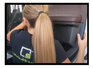
2. Once all the screws are removed you can take off the door panel using a panel tool. Be sure to not break any of the clips or mounting hardware. Pull panel away slowly and unplug any electrical connections.
