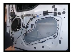
3. Now you are ready to prep the metal surface using a microfiber cloth, Acetone (use a breathing mask), and wipe away any moisture, oil, debris or etc. Then let air dry for an appropriate time. The point is to get the surface clean to ensure material glue contact.
