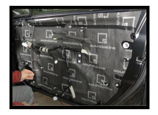
5. Locate the piece of the kit with the label on the back that coincides with the door you're working on. Make sure it lines up and is correct before you pull the white cover paper off. After you confirm the right piece, pull off the white paper and use a roller to apply the material at the top and work your way down. Use a razor blade or household needle to release air. Repeat for all door panels.
