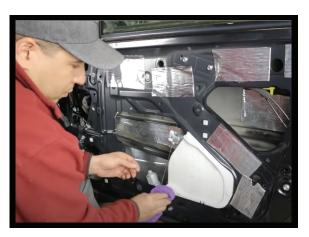
3. Now you are ready to prep the metal surface using a microfiber cloth and Acetone (or other cleaning solution). Wipe away any moisture, oil, debris, etc. Then, let it air dry for an appropriate time. The point is to get the surface clean to ensure material glue contact.
