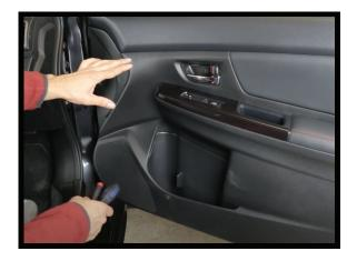
1. Start by locating the fastening hardware on the door panel. Take the appropriate screw driver and remove. Once all the screws are removed you can take off the door panel gently using a panel tool, watching that you don't break any of the clips or mounting hardware.
