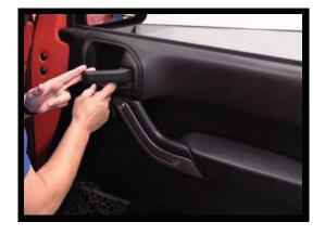
1. Start by locating the fastening hardware on the door panel, take the appropriate screw driver and remove.
