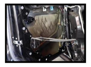
4. Next you need to prop the window up by either a rubber wedge or simply put a screw driver through the bottom hole as illustrated.
