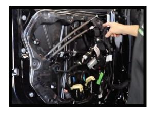
3. You will find an insert that needs to be removed, with mounting screws and cables that control door handle and locking mechanism. Slowly pull the insert away and pull through the cables to give yourself some slack.
