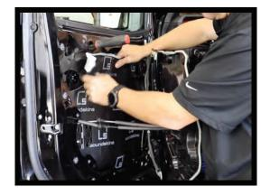
5. Now you are ready to prep the metal surface using a microfiber cloth, Acetone (use a breathing mask), and wipe away any moisture, oil, debris or etc. Then let air dry for an appropriate time. The point is to get the surface clean to ensure material glue contact.
