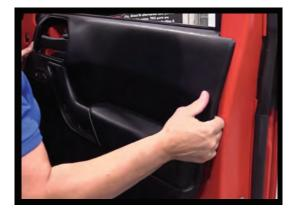
2. Once all the screws are removed you can take off the door panel gently watching that you don't break any of the clips or mounting hardware. Pull the panel away slowly and unplug any electrical connections.
