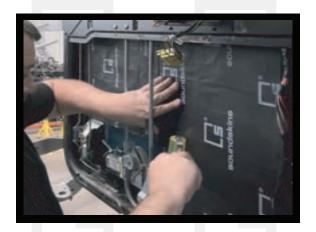
6. Make sure you window is rolled up. Take the outer door skin piece and ensure it aligns correctly. Then pull a couple inches off the left side of the piece, align it with the edge of the door, and tack the piece down. Apply from left to right with a roller, peeling off the backing paper as you go. Make sure the piece is pushed down evenly with no air bubbles.
