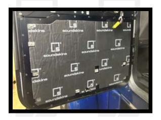
4. When the surface is dry and clean, locate the inner door skin piece. Make sure it lines up correctly before installing, then pull a couple inches of one side of the backing paper off, align it with its proper plugs and holes, then tack the kit piece in place. Apply the material from one side to the other with a roller, peeling off the backing paper as you go. Make sure the piece is pushed down evenly with no bubbles.
