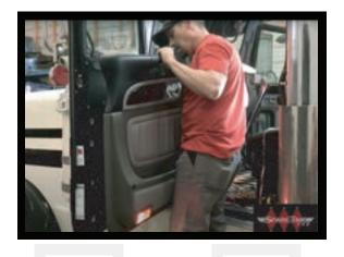
2. Use panel tool or hands to carefully pop up the plastic door panel and unplug the light cables. Slowly pull the door panel away and set it down to the side.
