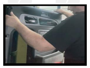
7. Replace the metal inner door skin panel and the plastic door panel, ensuring everything is installed properly.
