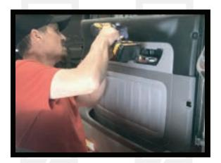
1. Start by locating the fastening hardware on the door panel, take your screw driver and remove. (T30 torx bit on side door grab bar, #3 screws on upper door grab bars, door handle, power switch, along the sides of the panels, some are covered by circular keepers that you need to pop out first) Use a panel tool to remove door handle plate.
