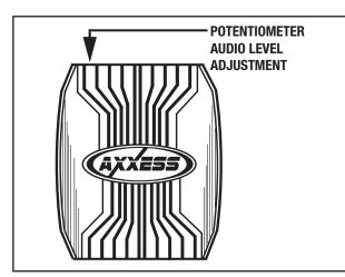
When using the CHTO-013 with a radio that has a high audio pre-out voltage, usually greater than 2 volts, the audio signal may become distorted. To resolve this follow these steps:
