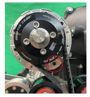
8) Lock the lateral position. The rear 3 bolts parallel to the tube should already be tight. First, lightly snug the upper center clamp bolt. Second, lightly snug the lower center clamp bolt. Third, lightly snug the 3 bolts parallel to the tube to remove any clearance between the clamp and the housing. Tighten the upper 3 clamp bolts. Tighten the 3 lower clamp bolts. Tighten the 3 bolts parallel to the tube.
