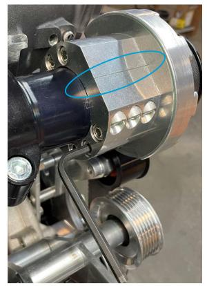
9) Align the shaft bearings. Remove the front cover and the belt. Install the dial indicator as shown to measure the adapter runout. We provide a .0005 indicator.
