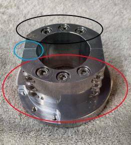
5) Slide the assembly onto the shaft housing, make sure it moves freely so you can align the belt window to your belt that is outlined in the next few steps.
