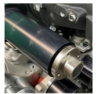
3) First, remove the front bearing support plate using the 6 small button head screws. Second, remove the front cover housing using the six M6 Socket Head Allen screws. The rest of the assembly does not need to be disassembled.
