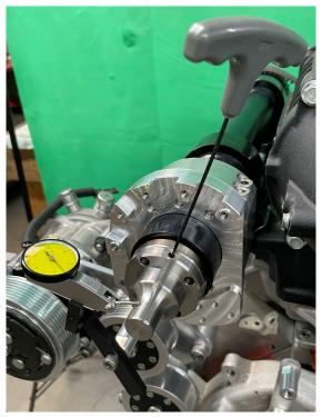
and tighten the M5 screws, once the pulley is installed re-check the runout to insure nothing has moved and remove one screw at a time and apply a small amount of blue Loctite to the screws and torque to spec ()
