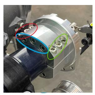
Once all the bolts have been tightened, torque to spec (see last Page)
