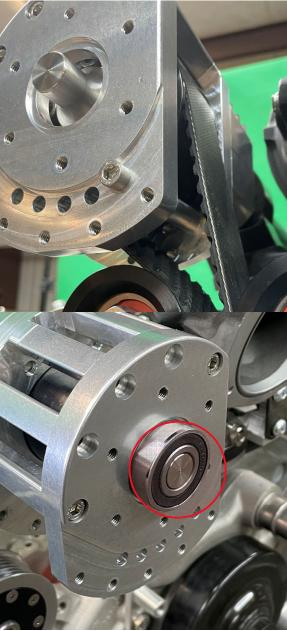
8) Lock the lateral position. first lightly snug the 3 bolts parallel to the tube to remove any clearance between the clamp and the housing (circled in blue) and then tighten the 3 bolts closest to the supercharger (circled in red) and finally tighten the 3 remaining clamp bolts facing the outside (circled in Green)
