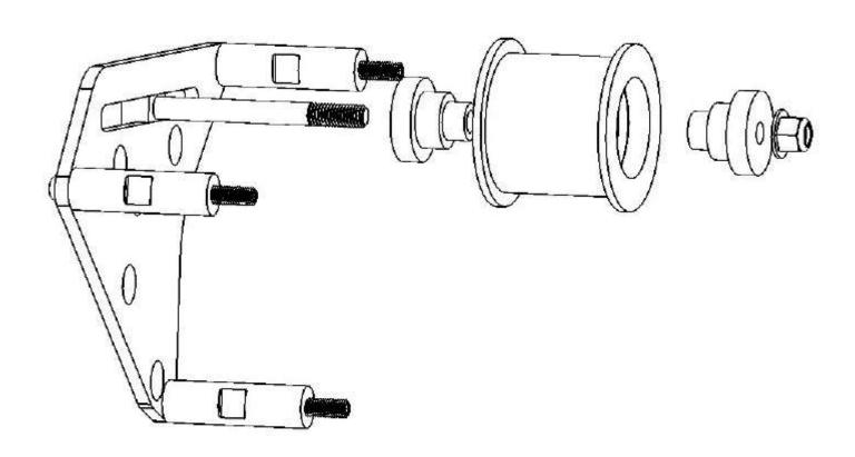
15: Install the belt with the 2.5" Smooth Idler Pulley to the inside of the belt
