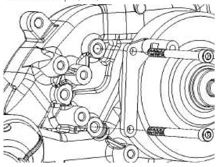
12: Assemble the *Rear Idler Plate* by attaching the three *Threaded Idler Plate Spacers with Studs* with two *8MMX20MM Button Head Allen Bolts* and one *8MMx20MM Flat Head Allen Bolt* as shown. Apply a small amount of blue Loctite to the bolts before assembly and torque to 12 ft. lbs
