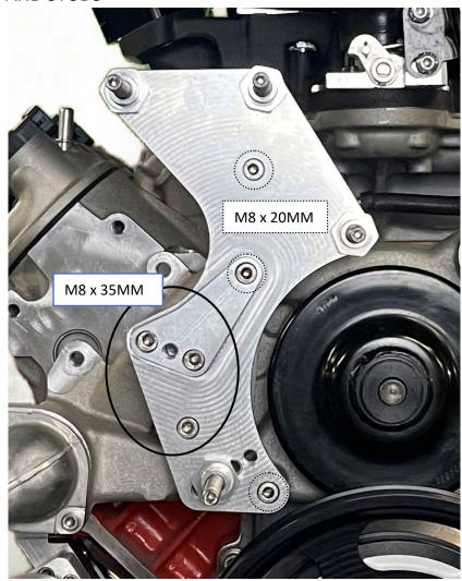
e) Install the <u>Pulleys</u> with snap rings facing outwards and install the outside (3) <u>Pulley Standoff Retention Nuts</u>. Apply a small amount of Anti-Seize to the threads and Torque to 20 ft. lbs.
