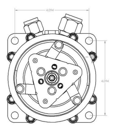
Partial List of Compatible A/C Compressor Part Numbers: Sanden 4514 (SD508 series), 4522 (SD508 series), 4665 (SD7 series), or 9537 (508 series), 047002-MUR (SD508 Series), 047007 (SD709 series)
