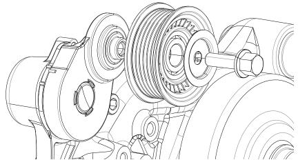
Compatible LSA Tensioner with pre installed 68MM Pulley
