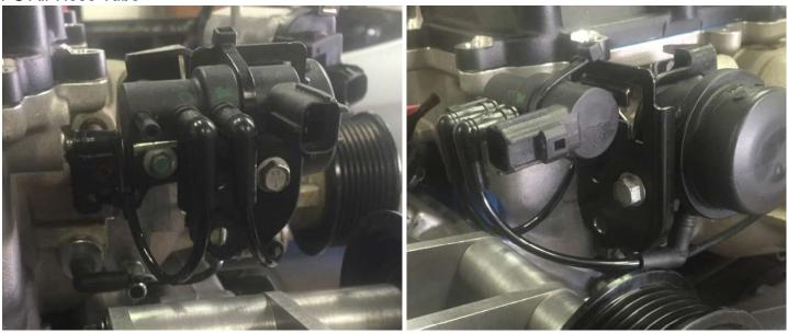
**Example 2:** this example is the same orientation as the last example but this one is shown using custom bent Stainless Steel 304 Capillary Tubing 4mm OD
