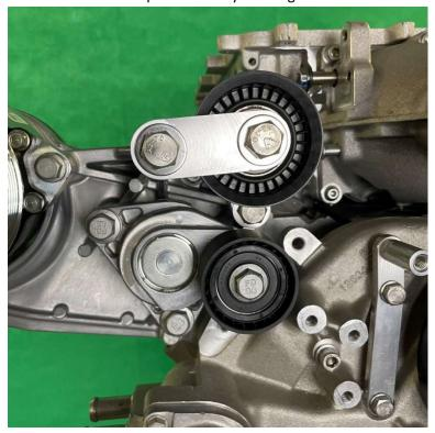
6. Install your serpentine belt and ensure the belt has the indicator on the tensioner arm is between the two indicators closest to full tension.
