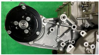
2. Using one of the M10x90MM Head bolts and a washer install the rear Support bracket with the short spacer in the upper bolt hole. Leave it slightly loose enough to move the bracket to align with the front bracket when it is installed.
