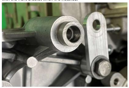
3. Bench assemble the front bracket using the long spacer M10x90MM bolt and the short M10x50MM bolt as shown
