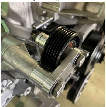
5. Install the Belt tensioner with the 50MM pulley that was included in your kit. Tighten down all the 10MM screws as per the Holley Kits original instructions.
