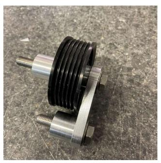
4. Install the front bracket onto the AC bracket aligning the small bolt with the original location of the idler pulley and the long bolt with the rear support bracket. And install the nylock lock nut on the back of the M10x90MM screw. You will need an open end wrench to tighten the lower M10 screw holding the rear support bracket.
