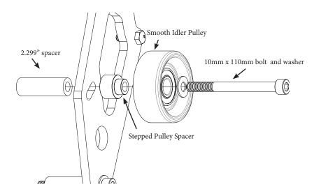
**Method 2:** Slide pulley/bolt towards the top of the slot
