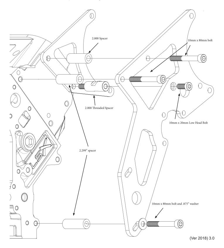
2: If your block has the upper mounting boss as shown the picture, mount the idler pulley using method 1, If your block does not have the mounting boss use method 2 for mounting your idler pulley
