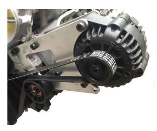
2.250" Spacer, 10mm x 110mm bolt, Stepped Idler Spacer and Idler Pulley
