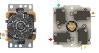
Connector on the Left follow the color when connecting conversion cable
