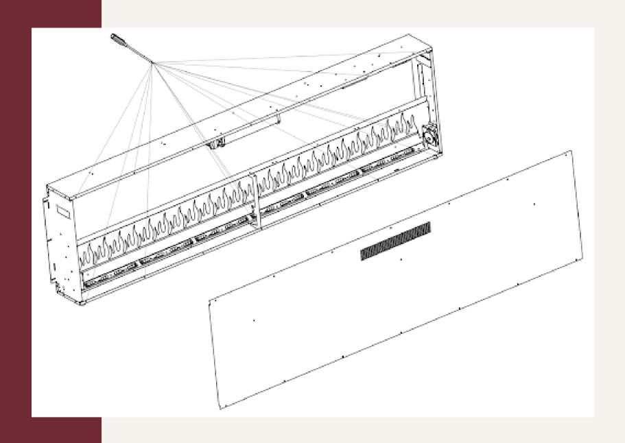
8 - 1 Remove the back panel of the fireplace by removing the screws surrounding the backplate.
