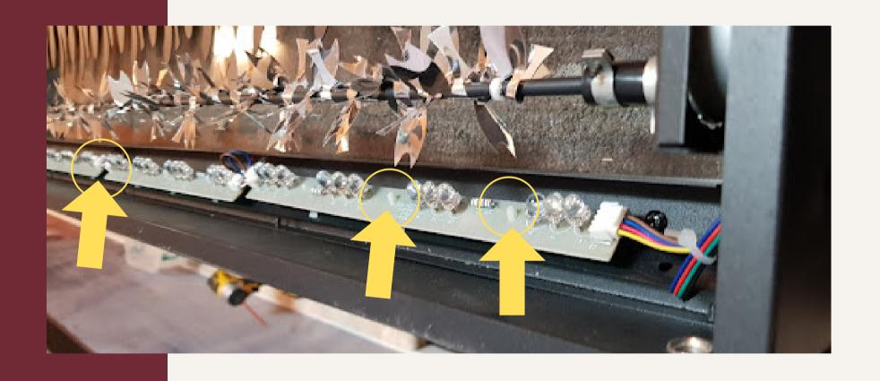
8 - 3 Squeeze the with pin and carefully pull the light bar up (Please do it one by one)
