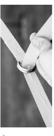
4. Feed the main line first through both rings then back between them and pull the tail until the HELP LINE is taut.
