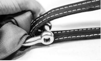
4. Screw the shackle pin hand-tight, DO NOT use additional tools to tighten shackle pin.
