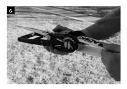
On the opposite tree, put the ratchet in the locked position and thread the other end of the webbing through the axle pulling until the line is taut. **IMPORTANT!** Pull the webbing through the axle by hand until it is as tight as possible and there is no slack in the line ("D" in Image 7). The ratchet can easily become over-spooled if the line is not pulled taut by hand first.
