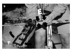
When this side of the webbing is fully tensioned, return ratchet to the closed, locked position. Check the ratchet to ensure it is locked so the bolt ("G" in Image 10 & 11) rests neatly in the cogging ("H" in Image 10 & 11) and the lever is in a fully closed, horizontal position parallel to the line ("I" in Image 11).
