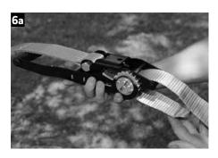
NOTE: It is especially important with Aggro Line or other power ratchets to thread the slackline into the axle slot from above with the ratchet handle facing the ground as indicated on the ratchet with an arrow (Image 6a). The extra bolt on these more powerful ratchets will prevent release if slackline is threaded incorrectly.
