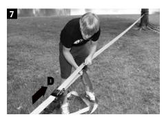
**IMPORTANT!** Pull the band through the axle by hand until it is as tight as possible and there is no slack in the band ("D" in Image 7). The ratchet can easily become over-spooled if the band is not pulled taught by hand first.
