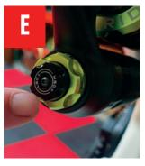
On the Öhlins equipped PRO model the black dial **(C)** is high speed compression and blue one is low speed compression **(D)**. For DVO equipped EXPERT models the compression is adjusted by a black dial on the top of the shock reservoir **(E)**.
