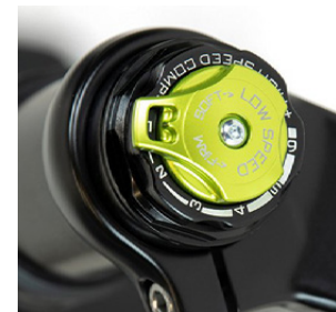
Above: DVO High Speed (black dial) and Low Speed (green dial) Compression Adjustment.
