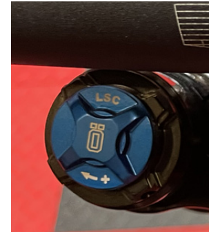
Above: Ohlins High (black dial) and Low Speed (blue dial) Compression Adjustment.
