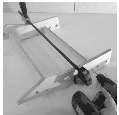
SIDE PANELS AND CROSS BATONS – CLAMPED STRUCTURE – CROSS BATONS IN POCKETS
