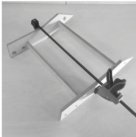
SIDE PANELS AND CROSS BATONS – CLAMPED STRUCTURE – CROSS BATONS IN POCKETS
