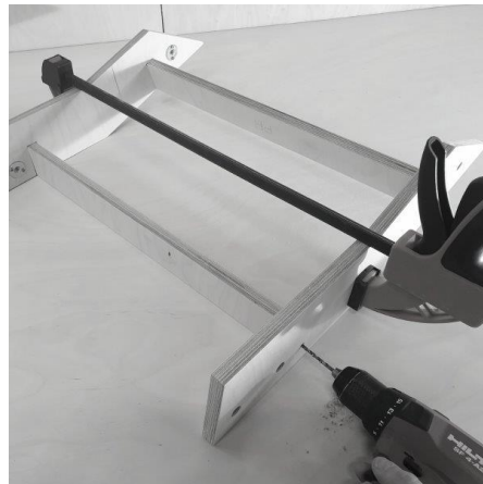
SIDE PANELS AND CROSS BATONS – CLAMPED STRUCTURE – CROSS BATONS IN POCKETS
