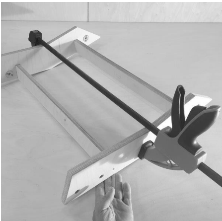
SIDE PANELS AND CROSS BATONS – CLAMPED STRUCTURE – CROSS BATONS IN POCKETS
