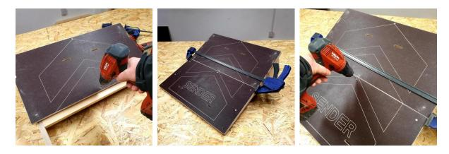
**Stage 10:**Drill through the two top marker points into the end of the side panels and fix with 2 No TX25 5 x 50 screws.
