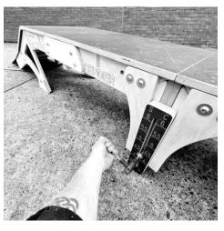
In this example we are adjusting the legs to match 500 mm HIGH RAMPS.
