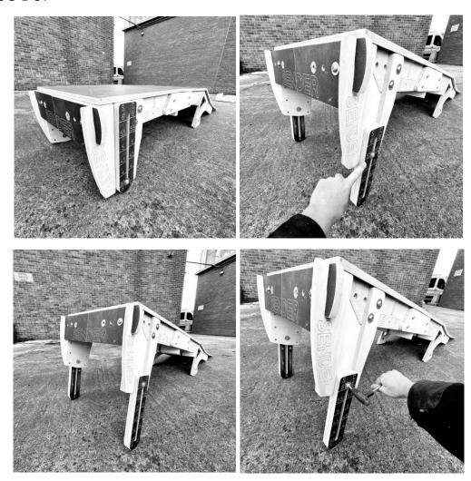
You may have to adjust the bolts at the join each time you increase the leg length because this changes the angle and relationship between the components.
