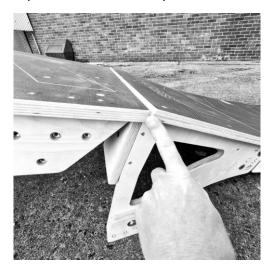
If you are connecting your Tabletop to a BIGGER RAMP like a 500 STRAIGHT RAMP. Hook the Tabletop to the Ramp first. The Legs will be at 350 mm. In this situation you have a DECLINED
