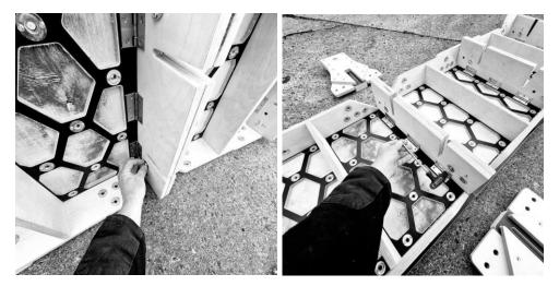
Take your Tabletop Legs and align them with the Tabletop sides and JOINED back plates. Use 4 x M10 x 40 mm Bolts with washers to secure the legs to the Tabletop. Tighten the bolts
