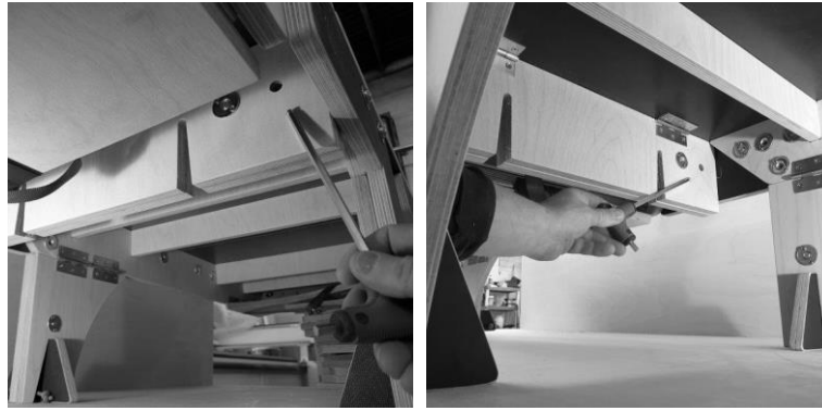
BOLTING TWO TABLETOP END PLATES TOGETHER
