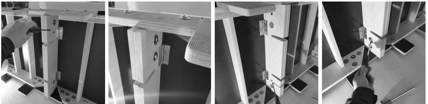
BOLTING TWO TABLETOP END PLATES TOGETHER
