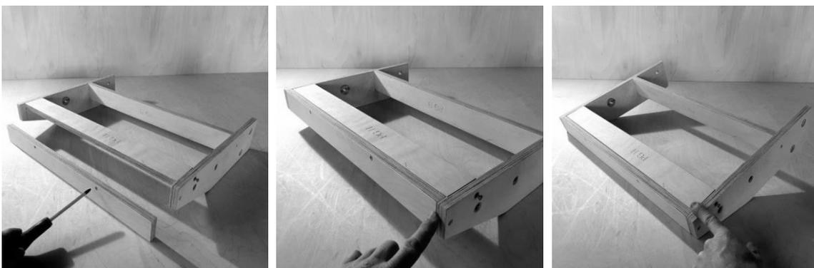
Drill through the marker points in V into H and fix with TX 25 Screws. You can now drive the screws completely into the end of H at both ends to trap PG V.
