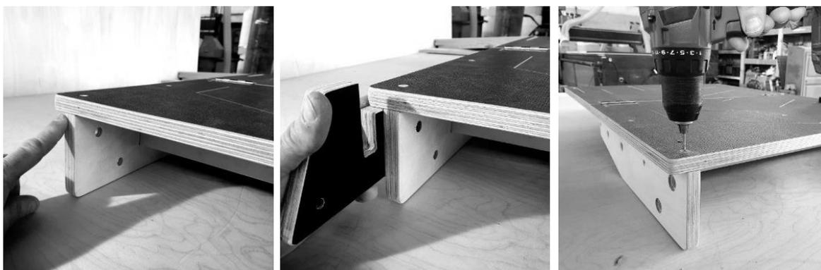
Now turn the structure around and repeat the process described above to SQUARE, DRILL and SECURE the Folding / Hinged end of the Surface to the Substructure
