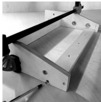
Take Component PG V and push / place this against PG H with the two marker points facing out as shown. IF PG V is a little loose then completely tighten the two screws above. A clamp can help to hold this component in place while you check the top and ends are flush.
