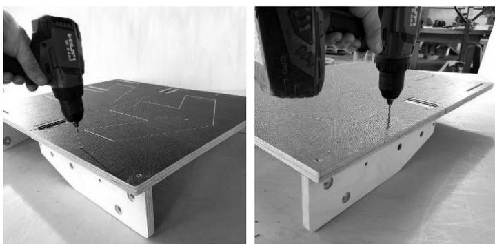
Turn the entire Structure over. You will see the 3 marker holes in Baton PG H. Place one of the 4 x 30 Stainless Steel Screws beside the drill bit and use a piece of tape on the drill bit to mark HOLE DEPTH. IF you drill too deep you will go through the SURFACE of the RAMP! The Drill holes should be 2 / 3 mm shorter than the Screw. Drill and Secure all 3 points with 4 x 30 Screws. Beware the Stainless Steel Screws are SOFT! Rounding the heads is possible if you DO NOT apply constant pressure.
