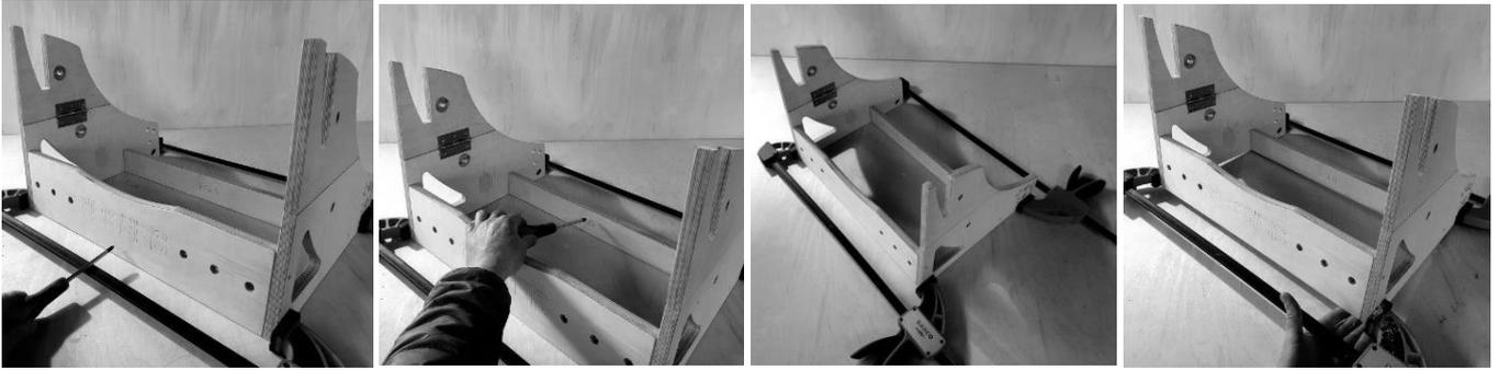
Drill through the Side Panels at the marked points into the ends of PG B and the Back Plate on both sides and secure with TX25 Screws.
