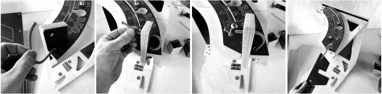
Repeat the process above on the other side to attach the Curved Leg and the Foot either FIXED or REMOVABLE
