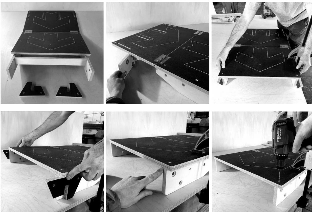
You may wish to rotate the structure. Follow the same process of checking with the block and ensuring the end of the surface and vertical end of the side panel are flush before drilling and securing with a TX25 Screw. It can be done without rotating the structure. Please see the example below.
