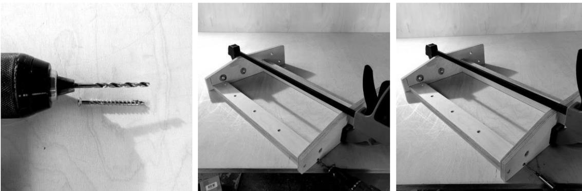
**\*\*Secure with a TX25 Screw LEAVING 15 mm PROTRUDING. As shown below\*\***
