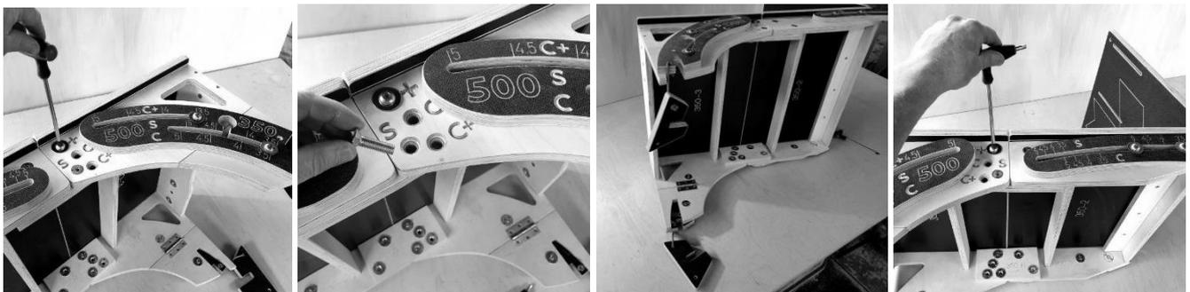
Repeat the process of loosening, sliding and then securing the bolts on the FRONT and REAR Curved Legs at the 350 C+ (OR 500 C+) marker lines. Loosen the + Bolt and remove the Bolt at position S. Manipulate the Sections so the C+ Hole lines up with the plate below and replace the Countersink Bolt by hand and then tighten the bolt.
