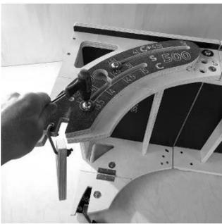
On the Curved REAR LEG ensure the 350 S (OR 500 S) Marker line is central with the SECOND BOLT then tighten both bolts to (12 Nm). **TURN THE RAMP OVER** and align the second Joining Plate repeating the process above so the permanent fixing points are secured BEFORE adding the Button Head Bolt and Washer to the + Hole. Manipulate and Align the hole so you can place an M10 x 35 Countersink bolt by hand into the S Hole and wind this into the T Nut. Set BOTH front and REAR Legs as described above.
