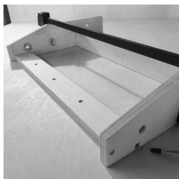
Drill through the side panel into the end of B on both sides and secure with a TX25 Screw. Rotate the structure and drill into the other end of H.
