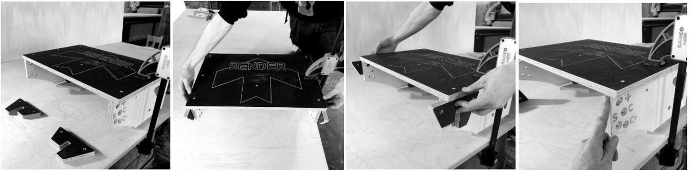
You may wish to rotate the structure. Follow the same process of checking with the block and ensuring the end of the surface and vertical end of the side panel are flush before drilling and securing with a TX25 Screw.
