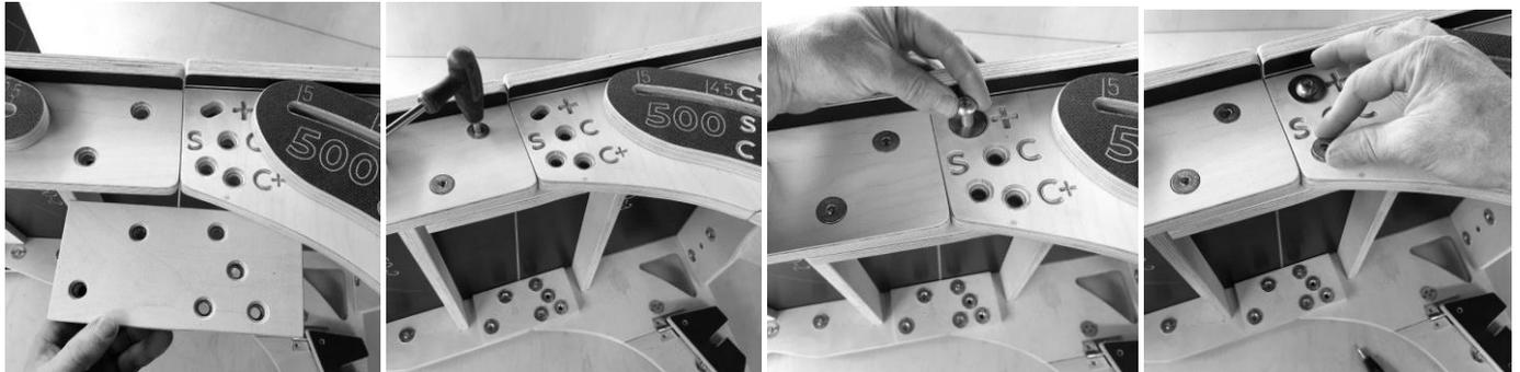
If the feet have been removed install / push these into place before turning the ramp over into JUMP MODE. Go around ALL the ramp bolts checking that they are tight before starting a JUMP SESSION. You are now ready to TAKE OFF or LAND at ADVANCED 350 STRAIGHT. OR if you have an EXPERT RAMP it will be 500 STRAIGHT.
