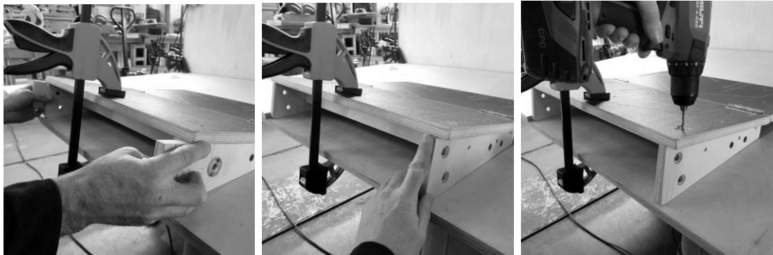
CLAMP THE RAMP SURFACE AND SUBSTRUCTURE TO THE TABLE AND USE THE 200 L / R BLOCKS AS SPACERS
