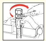
Step 4. Male Ends: Screw nipple clockwise into socket and hose. Leave a 1/32∀ clearance between nipple hex and socket.
