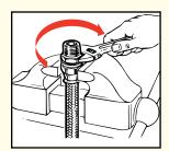
Step 4. Wrench tighten hex until clearance with socket hex is at .031 inches. Your thumbnail is a convenient measuring device. Tighten further to align corners of nipple and socket hexes. CLEAN, PROOF TEST TO TWICE OPERATING PRESSURE AND INSPECT ALL ASSEMBLIES.
