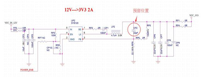
Figure 12 The DC-D C antihypertensive circuit diagram
