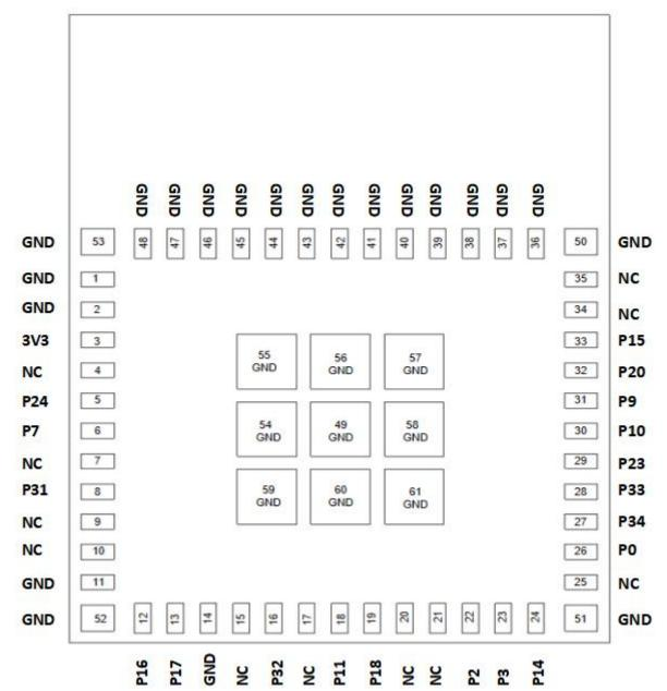
Figure 5 Schematic diagram of module pins(top view)
