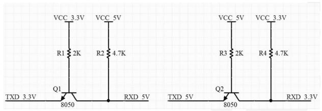
Figure 13 Level convert circuit
