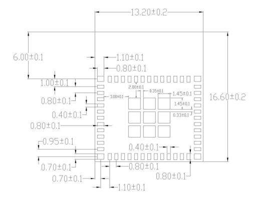
Figure 4 Module size diagram
