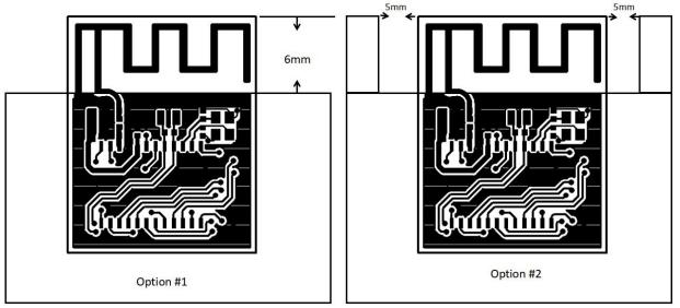
Figure 11 Schematic diagram of the antenna layout
