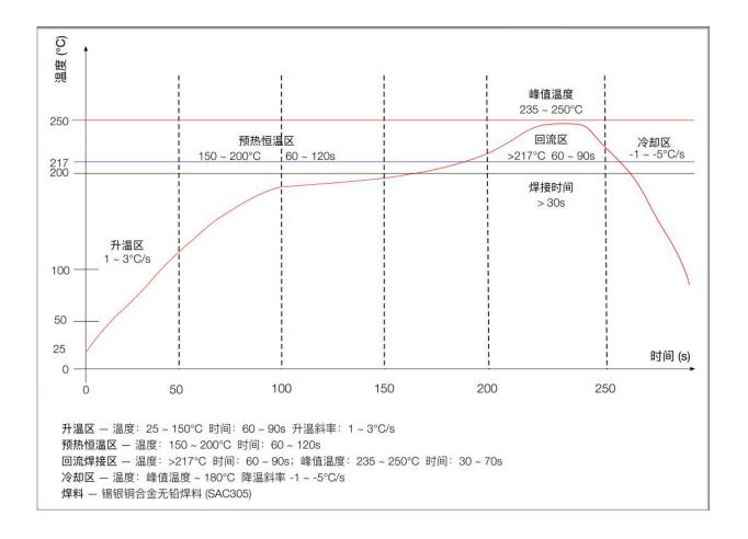
Figure 14 Flow welding diagram
