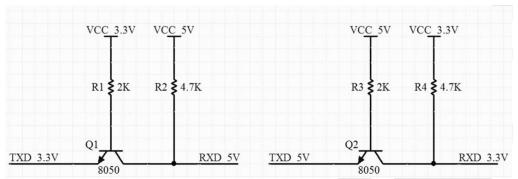
Figure 16 Level switching circuit
