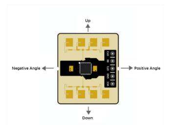
Figure 13 Schematic diagram of gesture recognition detection range
