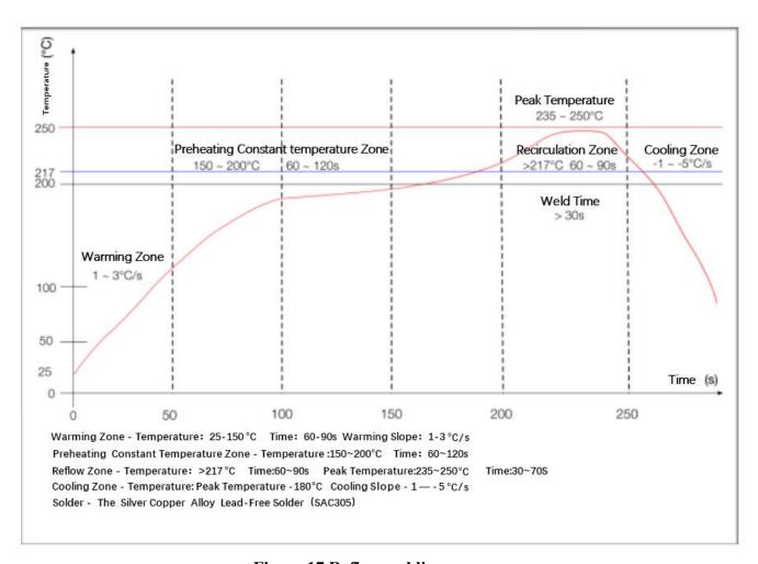
Figure 17 Reflow welding curve
