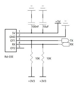
Figure 7 Application guide circuit
