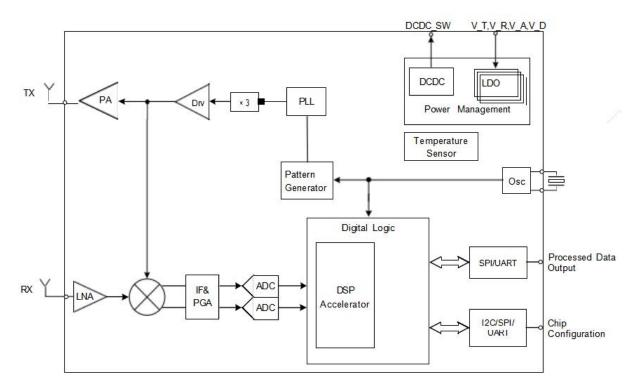
Figure 1 S3KM111Larchitecture diagram
