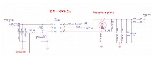
Figure 15 DC-DC step-down circuit diagram
