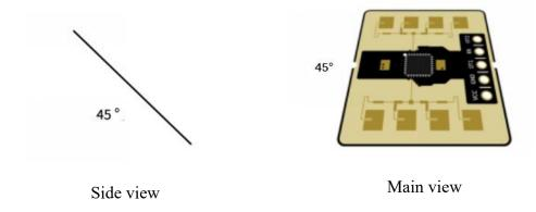
Figure 12 Schematic diagram of tilted installation for gesture recognition
