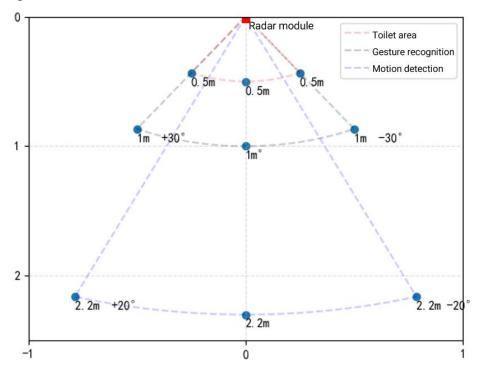
Figure 14 Gesture recognition hanging wall radar power diagram
