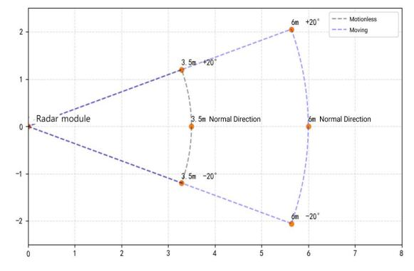
Figure 11 Power map of precision ranging wall-mounted radar
