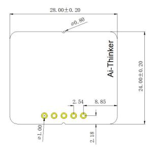
Figure 8 Recommended PCB package size
