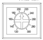
**Note:** To protect the motor, set the arrow number as the same as the motor nominated power. Whenever overload occurs the drive will turn out to be the protection mode.
