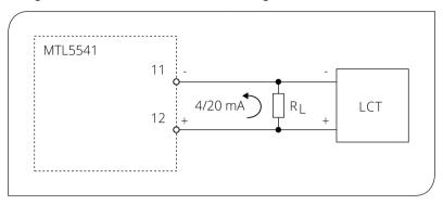
Configuration B:  $180 \Omega \le RL \le 580 \Omega$  (using the internal resistance)
